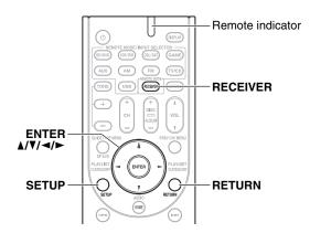
The on-screen setup menus appear on the connected TV and provide a convenient way to change the AV receiver's various settings. Settings are organized into 10 categories on the main menu.
